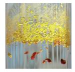
The iron(II) complex  $[Fe(L)_2](BF_4)_2$  [L=2,6-bis(1H-pyrazol-1-yl)-4-(thiocyanatometh-yl)pyridine] displays polymorphism in the solid state: it can be obtained in two crystalline forms at room temperature, from the same solution and side-by-side. One (yellow) has the molecules in a high-spin state that is virtually independent of temperature, whereas the other (red-brown) shows spin-crossover behaviour.
